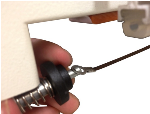
Figure 5. Attach other end of element to the spring hook assembly at the front of the sealing arm.
