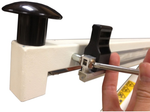
Figure 6. Unscrew the silicone bracket and remove screw, washer and spacers.
