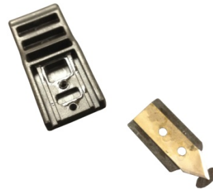
Figure 9. Carefully remove the old blade.
